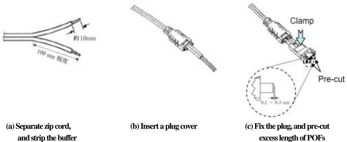
Figure 18: An example of setting and termination process of a POF connector [11]
