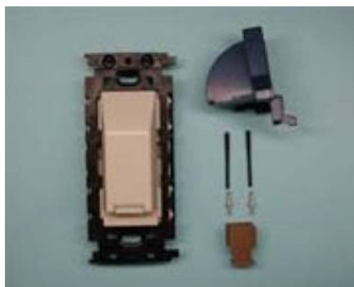
Figure 15: An example of telecommunication outlet for duplex fluoropolymer-type POF [9]
