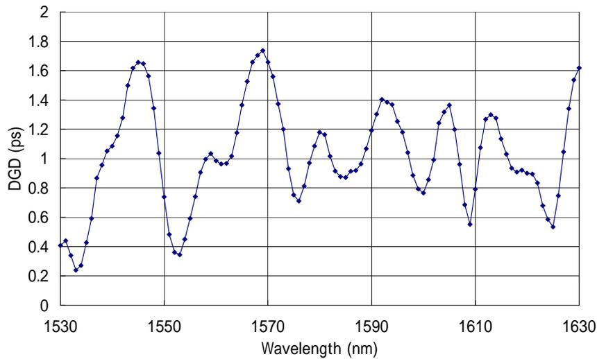
Figure 2 - DGD versus wavelength for a random mode coupling device (example)
