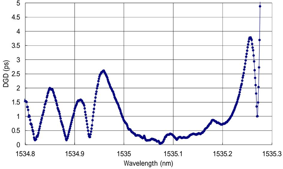
**Figure 3 - DGD versus wavelength for a fibre Bragg grating filter (example)**
