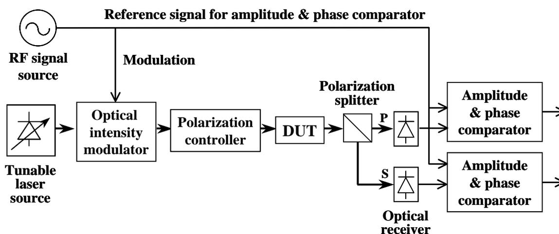
Figure 1 - Block diagram for polarization phase shift method
